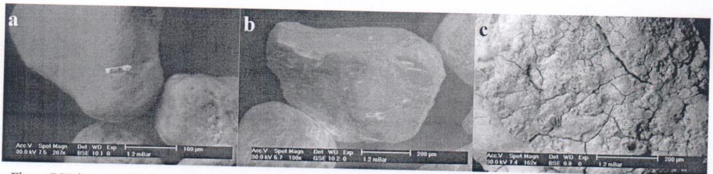
Fig. 5: BSE images of (a) goethite completely altered to uraninite (sample Z29), (b) uranophane strongly replaced by torbernite (sample Z29) and (c) autunite with cracks as a result of dehydration process (sample Z41)
